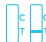
**10** Test result is displayed 15-30 minutes after the liquid is expelled into the well. After 30 minutes, the result is invalid.
