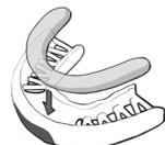
Pack the Zone Fit Material into the top side of the frame.
