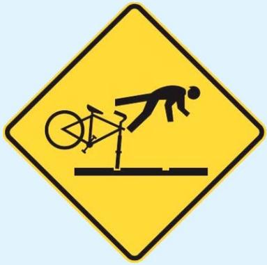
Cyclists should be aware of tram tracks at intersections and other areas. The groove in the tram tracks may cause a bicycle's wheel to become stuck if the cyclist rides parallel to the tracks. Cyclists can safely cross tram tracks by approaching at right angles.
