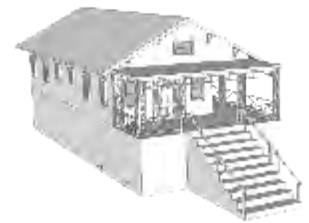
Lift the entire house, with the floor slab attached, and build a new foundation to elevate the house.
