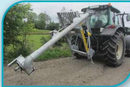
A slurry agitator is used to agitate (mix) slurry which is kept in a tank or pit on the farm.
