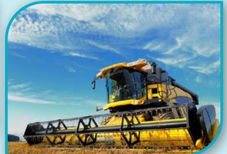
The header on a combine is powered with a P.T.O.
