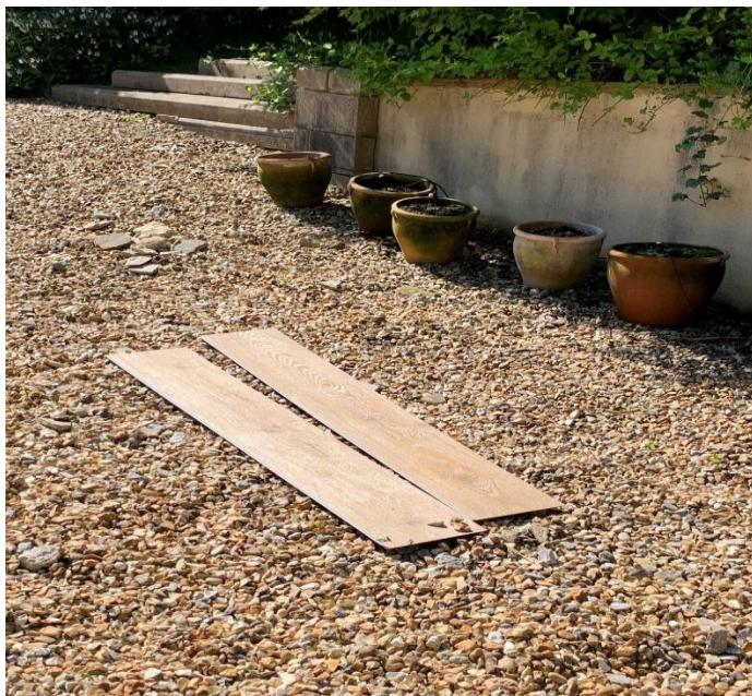
The two boards - placed on a gravel driveway last July - were left exposed to the soaring temperatures of Summer 2019 which then quickly changed to a wet and harsh winter, with the boards at some points even being covered in snow.
