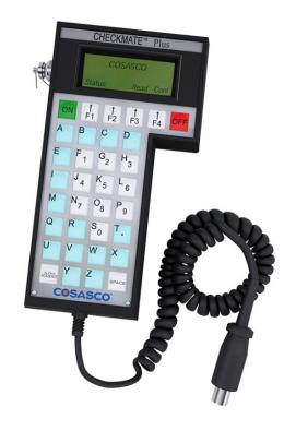
The Checkmate Plus Electrical Resistance (ER) Instrument uses "state of the art" surface mount integrated circuits, the sophisticated electronics provides higher resolution and measurement accuracy of ER probes. The measurement cycle time for direct probe readings has been reduced to 30 seconds while still maintaining high accuracy.
