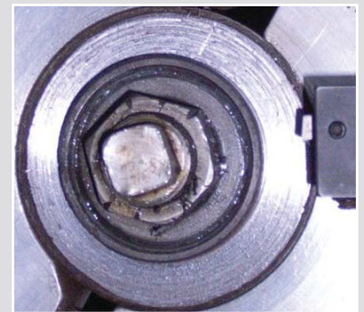
Access Fitting after re-facing
