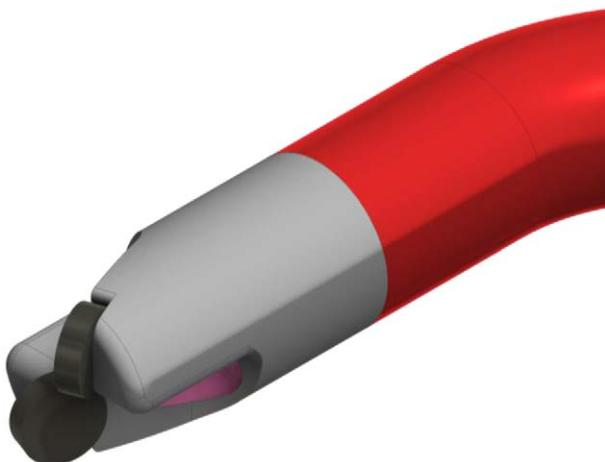
Figure 13—The drill bit with a needle bearing connection with the micro-casing
