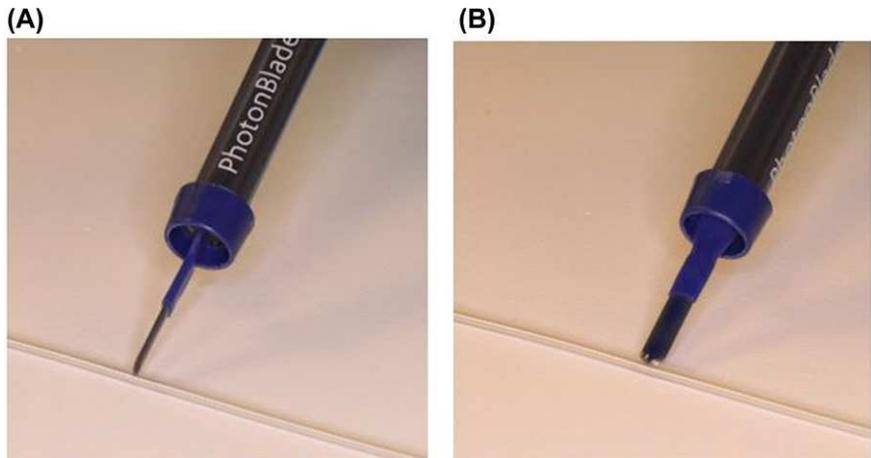
**FIGURE 1** Blade orientations. Panel (A), perpendicular active edge (active) blade orientation; Panel (B), parallel flat blade (flat) orientation [Color figure can be viewed at [wileyonlinelibrary.com](http://wileyonlinelibrary.com)]
