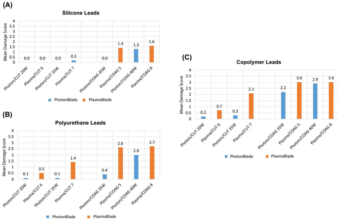
**FIGURE 3** Phase 2 Mean damage scores by lead insulation material. Panel (A), silicone; Panel (B), polyurethane; Panel (C), copolymer [Color figure can be viewed at [wileyonlinelibrary.com](http://wileyonlinelibrary.com)]**TABLE 5** Rates of damage by device for matched settings
