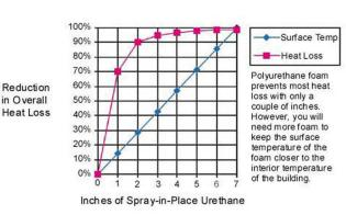
insulation is added to the surface temperature. In other words, by super insulating, the surface temperature of the inside of the exterior walls comes very close to the room temperature. This prevents condensation, which prevents the growth of mold.
