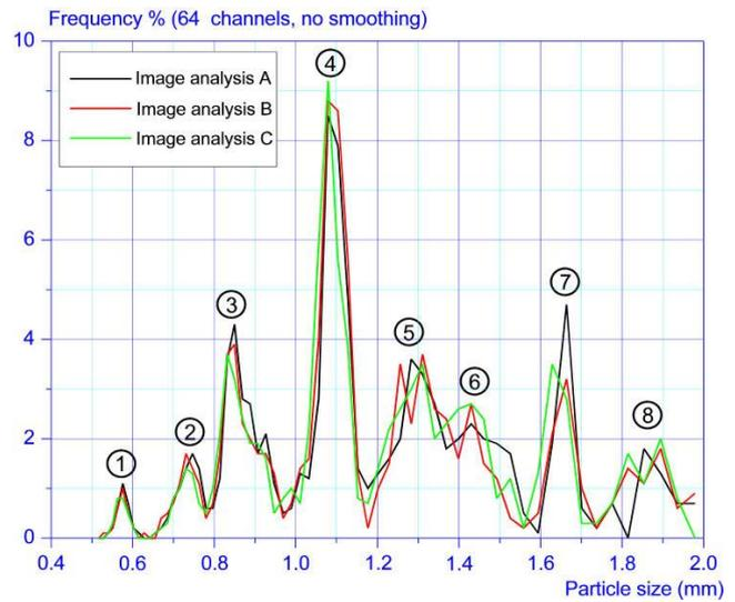
Fig 1. Microscope Analysis of a 500-2000µm IA Standard
