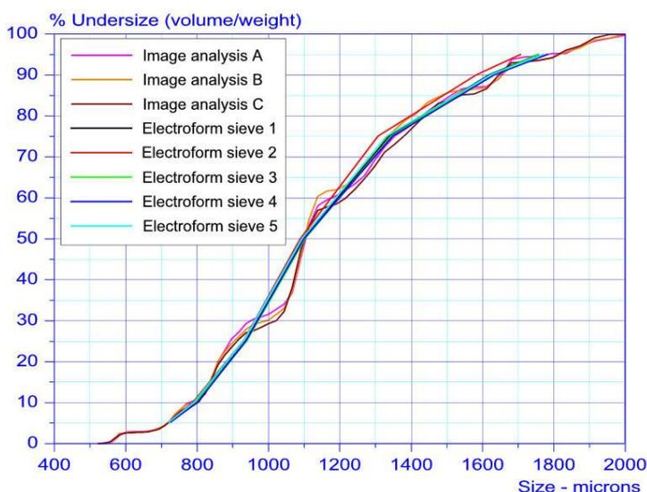
Fig 2. Comparison of Image Analysis and Sieve data for a 500–2000µm IA Standard
