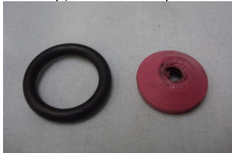
X884 (88-21 O-ring, 418-B Beveled Washer)
