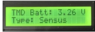
Battery Voltage Indication
