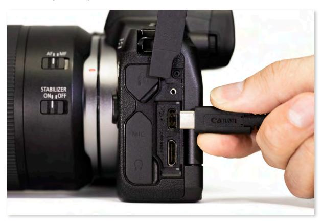
**14.** Turn camera on. It is recommended to use Movie Mode. Set this with your camera's Mode Dial, Mode Switch or Mode Button interface. Note: If EOS Utility opens, quit the program completely.
