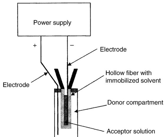
Fig. 1. Schematic illustration of the equipment for electro membrane isolation (EMI).
