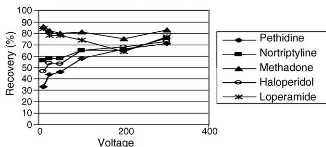
Fig. 5. Effect of voltage on cross-membrane transport recovery versus EMI voltage).
