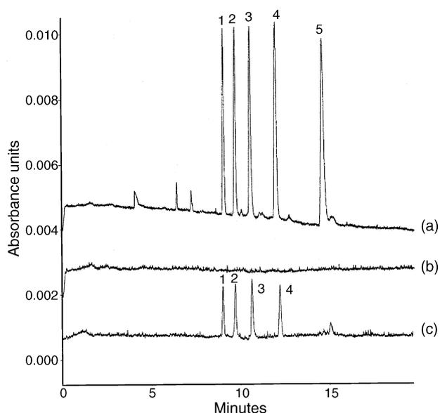
Fig. 3. Electropherograms demonstrating the strong effect of voltage on cross-membrane transport: (a) acceptor phase after 5 min of EMI at 300 V; (b) acceptor phase after 5 min of extraction with no voltage and with pH 2 in both the sample solution and in the acceptor (passive diffusion); and (c) acceptor phase after 5 min of extraction with no voltage and with pH 13 in the sample solution and pH 2 in the acceptor (passive diffusion).
