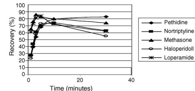
Fig. 4. Effect of time on cross-membrane transport (recovery versus EMI time).
