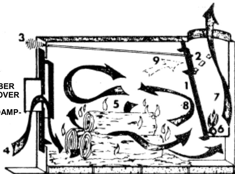
**CROSS SECTION ILLUSTRATING FUNCTION OF BAFFLE AND BAFFLE BYPASS**
