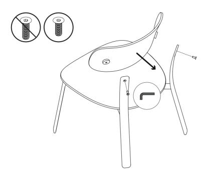
5. Fix the back rest of the SPRINGBACK lounge chair with M6X16 screws (short screws).
