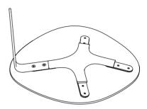
2. Screw the front legvs with M6X20 screws (long screws).
