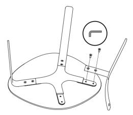
3. Screw the rear legs with M6X20 screws (long screws).
