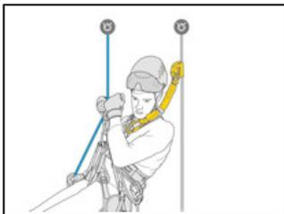
The ASAP'SORBER AXESS allows the rope to be kept at a distance to protect it during certain work phases.
