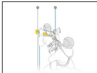
The ASAP'SORBER AXESS can be used for loads up to 250 kg in two-person rescue situations.
