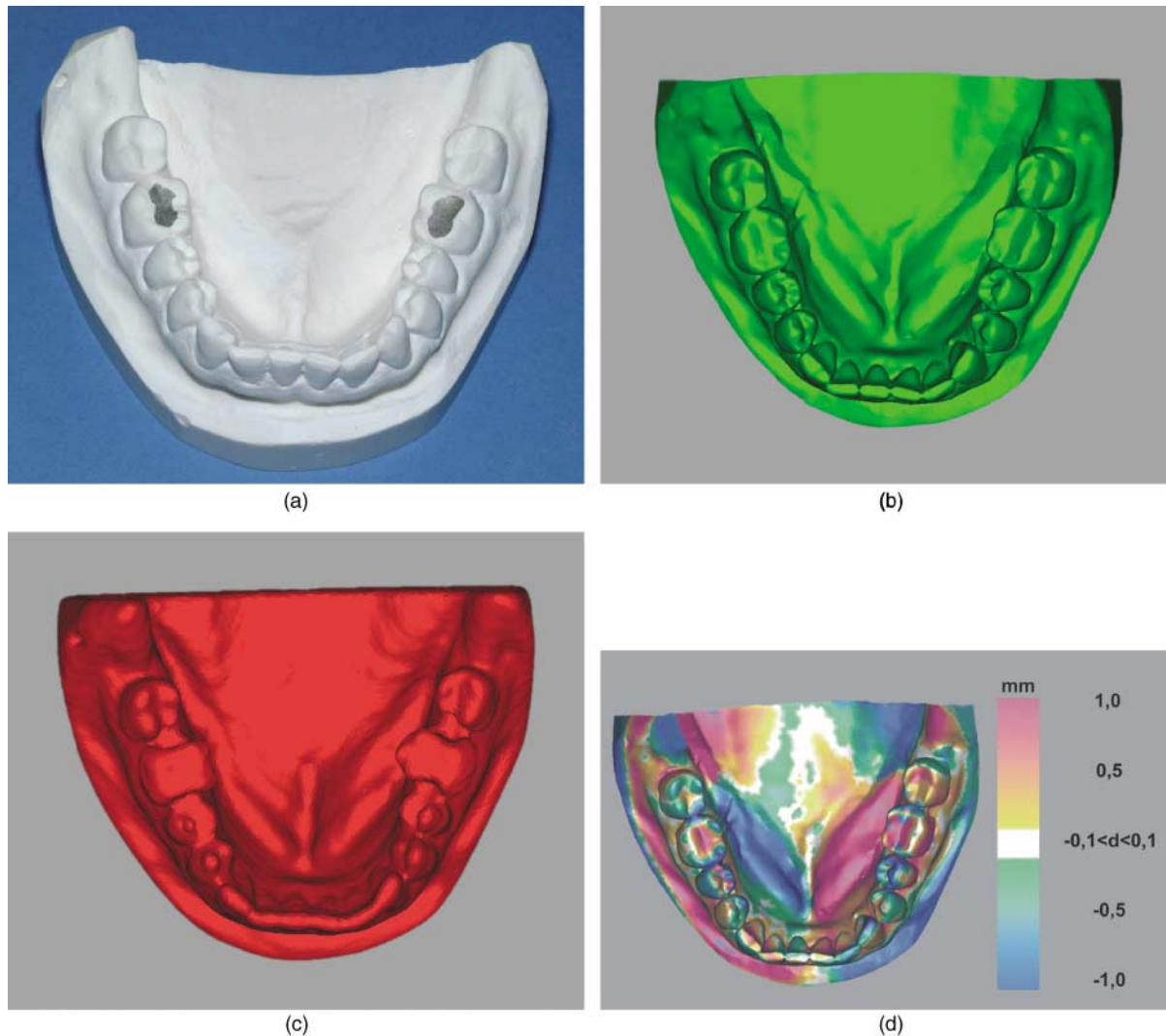
Figure 1 (a) Plaster cast with occlusal metal restorations in the first molars, bilaterally. (b) Optical surface data of the plaster cast. (c) Isosurface generated from the CT scan of the plaster cast after streak artefact correction. (d) Colour-coded visualization of the differences between CT and optical data after the registration procedure
