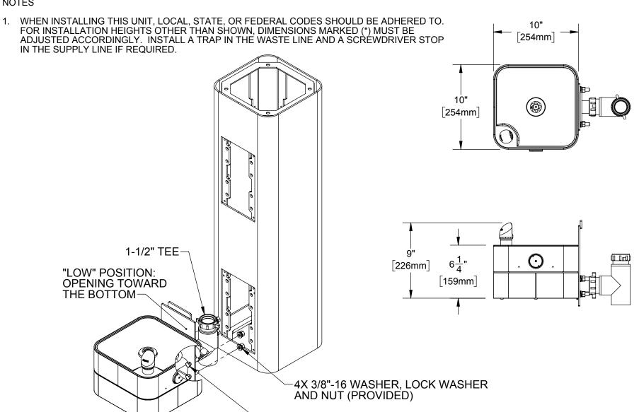
NOTE: STANDARD CONFIGURATION FOR MODEL 3670 ON A PEDESTAL IS SHOWN. IT IS RECOMMENDED THAT THE ASSEMBLY IS PLACED AT THE LOWEST OPENING ON THE PEDESTAL. THE MOUNTING PLATE CAN BE ROTATED SO THE DOG BOWL CAN BE IN A "HIGH" OR "LOW" POSITION. IT IS RECOMMENDED TO USE THE "LOW" POSITION AS SHOWN.
