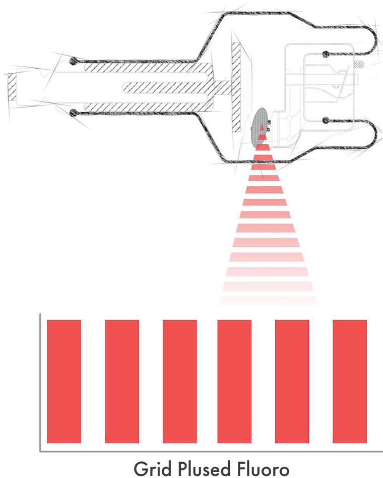
Figure 4 - Grid controlled X-ray tube
