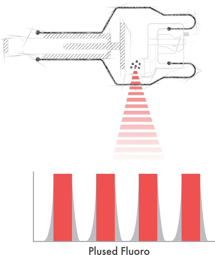
Figure 3 – Pulsed fluoroscopy using generator-controlled pulses
