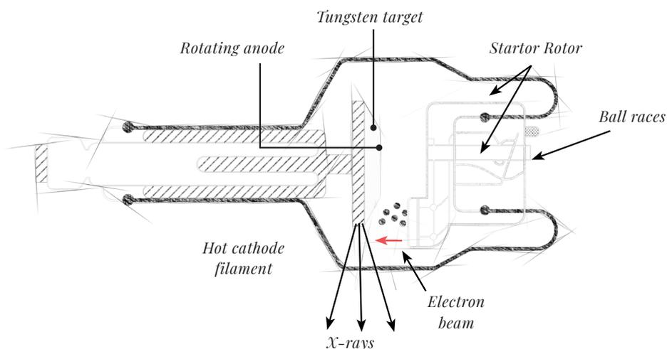
Figure 1 - Basic X-Ray tube
