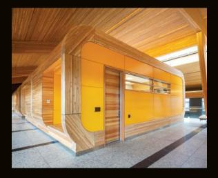
Westdek™ is manufactured to the same high standards as glulam and is guaranteed to possess the same long-standing history of durability. This product combines structural capacity with an attractive finish and can be used as a roof or floor panel.
