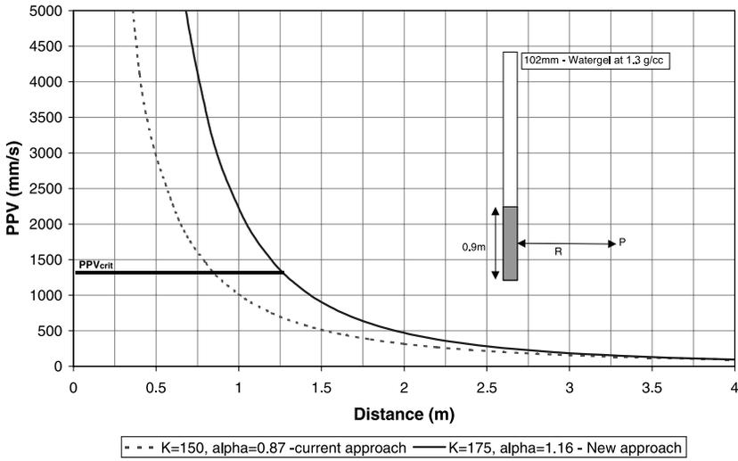
Fig. 16. Comparison between PPV attenuation – case study 4.
