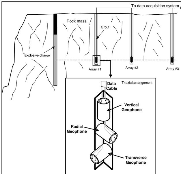
Fig. 2. Typical instrumentation layout for near field vibration attenuation monitoring in a pre-defined direction.
