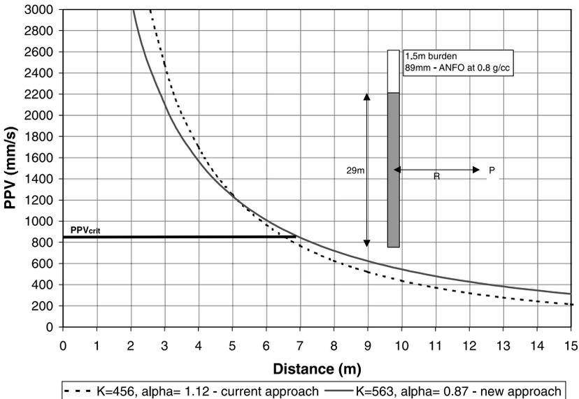
Fig. 12. Comparison between PPV attenuation – case study 2.
