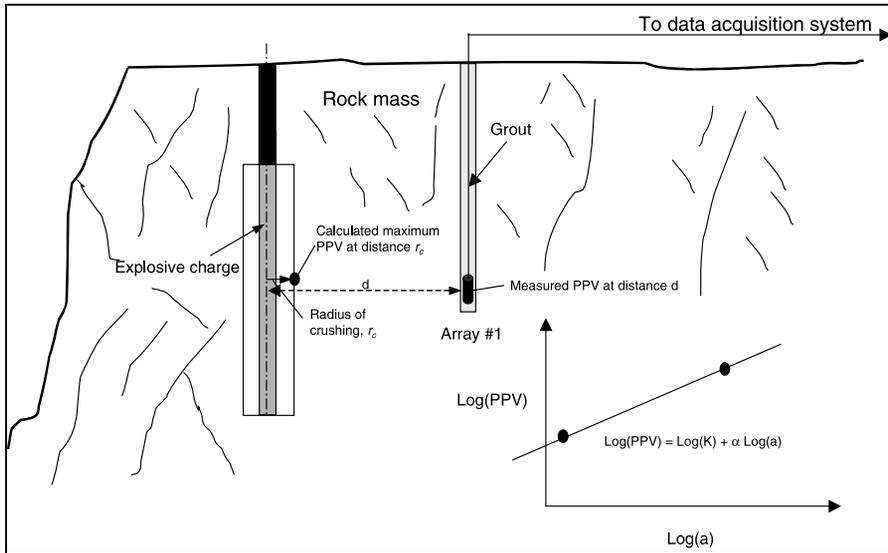
Fig. 4. Schematic diagram of new approach required to define the Holmberg–Persson attenuation constants.
