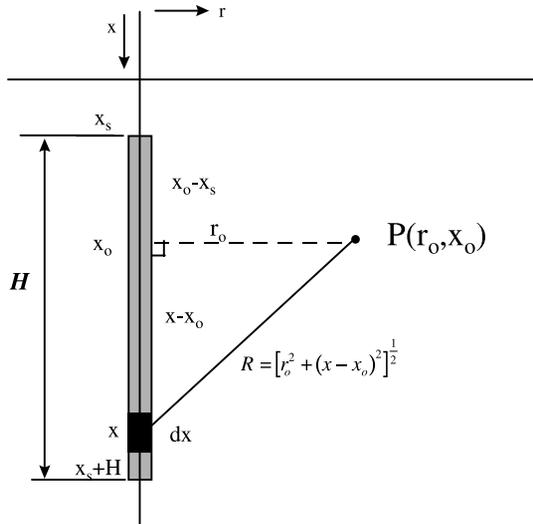
Fig. 1. Schematic diagram of the Holmberg-Persson parameters to model peak particle velocity attenuation.
