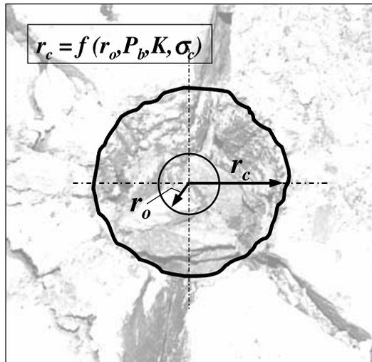
Fig. 6. Parameters influencing the extent of crushing.
