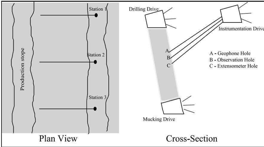
Fig. 11. Schematic diagram of stope instrumentation at Hilton/MIM.
