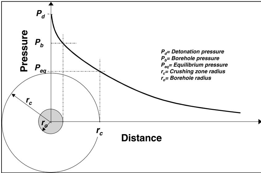
Fig. 5. Diagram describing pressure attenuation with distance.
