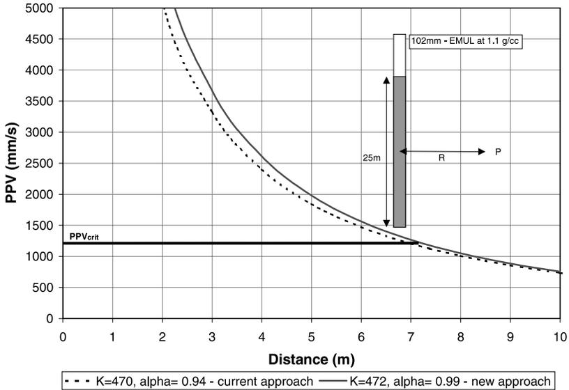
Fig. 14. Comparison between PPV attenuation – case study 3.
