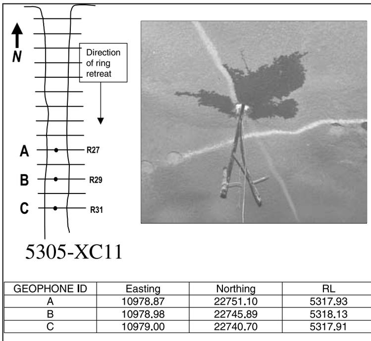
Fig. 13. Schematic diagram of monitoring layout.
