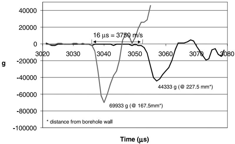
Fig. 9. An example of a typical acceleration signal from Test #1 [20].
