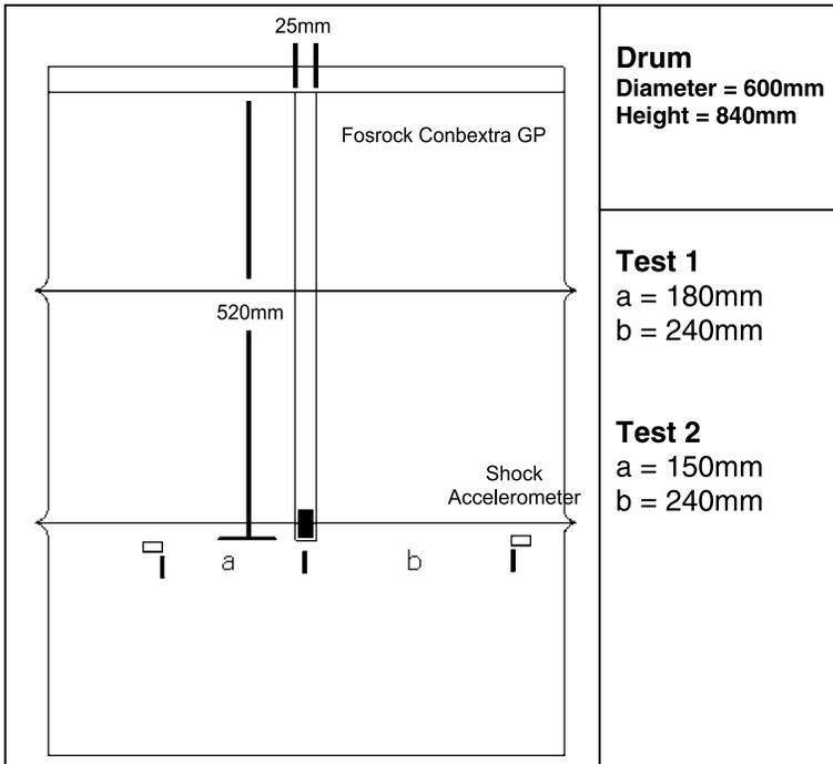
Fig. 7. Experimental set up [20].
