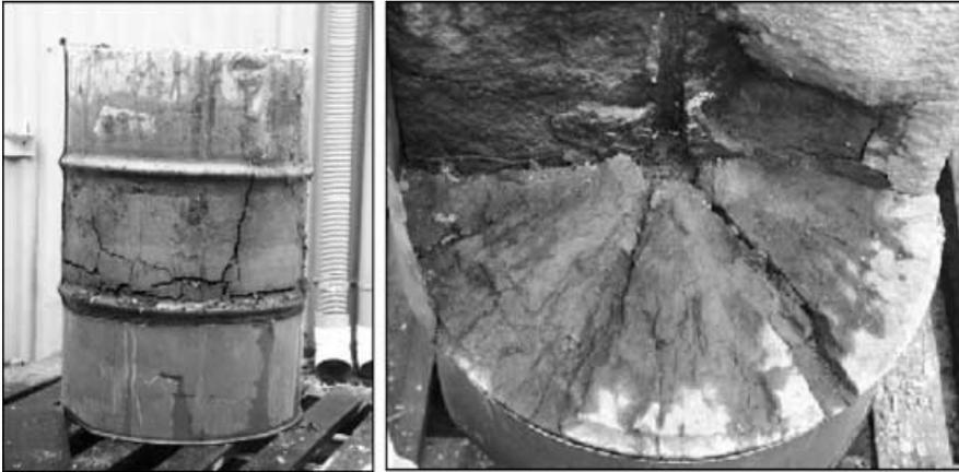
Fig. 8. Radial cracks and crushed zone measurement for Test #2 [20].
