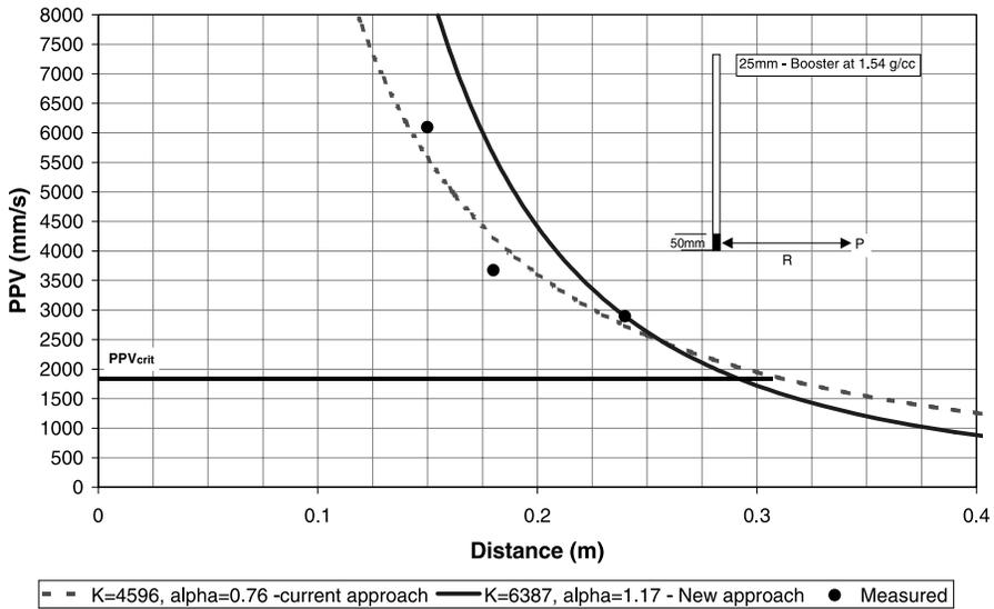
Fig. 10. Comparison between PPV attenuation – model scale tests.
