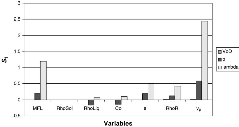
Fig. 8. Response of the sensitivity  $S_1$  to changes in the detonation parameters for Lee's (1990) emulsion
