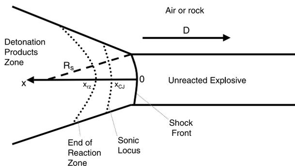
Fig. 2. Detonation front regime for non-ideal cylindrical explosive (Braithwaite et al., 1990)
