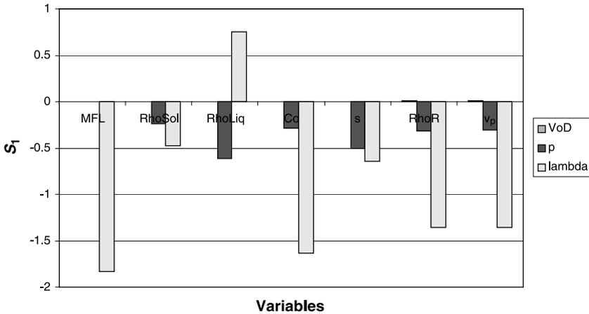
**Fig. 7.** Response of the sensitivity  $S_1$  to changes in the detonation parameters for Blend1
