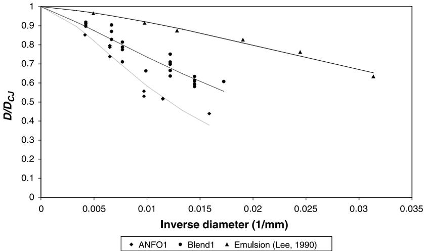
Fig. 5.  $D/D_{CJ}$  versus inverse diameter relations for the explosives included in the sensitivity analysis
