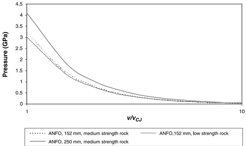
**Fig. 11.** The results of the Taylor wave model for ANFO confined in low (kimberlite) and medium (breccia) strength rocks at 152 and 250 mm diameter blastholes
