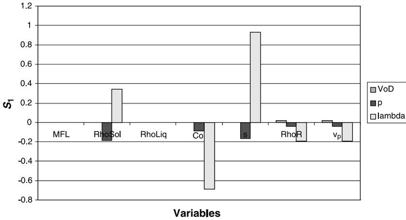
**Fig. 6.** Response of the sensitivity  $S_1$  to changes in the detonation parameters for ANFO1. RhoSol:  $\rho_S$ ; RhoLiq:  $\rho_L$ ; RhoR:  $\rho_r$
