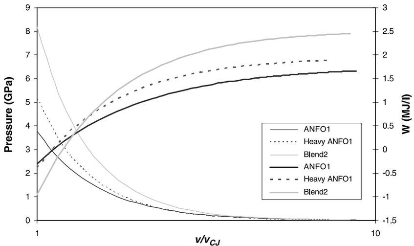
**Fig. 12.**  $p-v$  curve and the work done by the detonation products for ANFO1, Heavy ANFO1 and Blend2. Thin and thick lines represent the pressure and expansion work curves respectively for each explosive type
