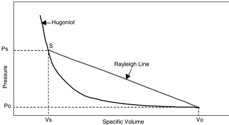
Fig. A.2. Typical  $p-v$  Hugoniot for an unreacted explosive (Cooper, 1996)
