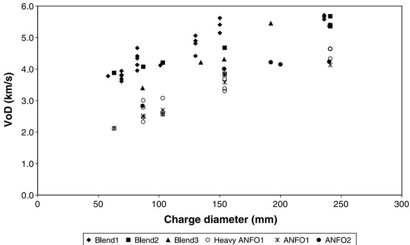
Fig. 4. Unconfined VoD versus charge diameter (Esen, 2004a)
