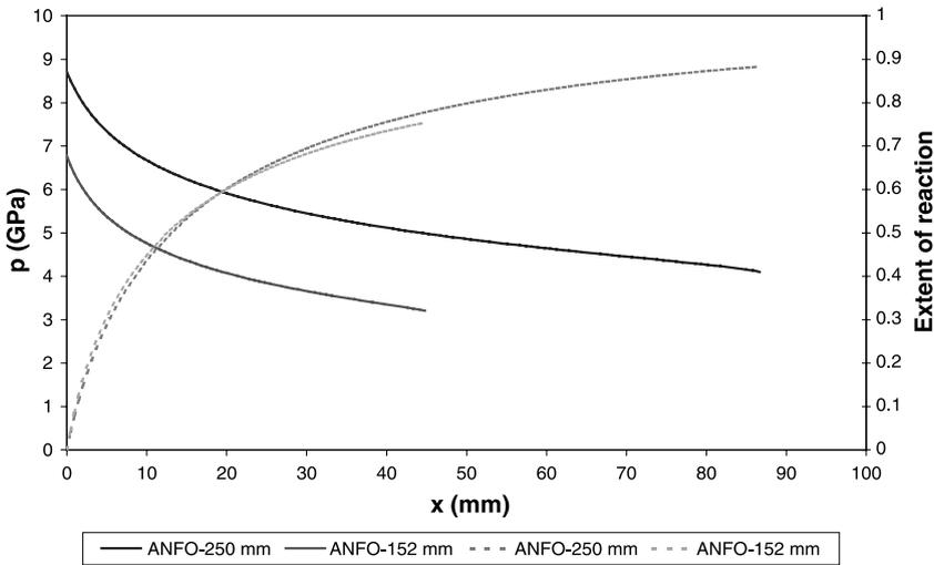
Fig. 9. Pressure and extent of reaction histories of ANFO at 152 and 250 mm in Breccia confinement
