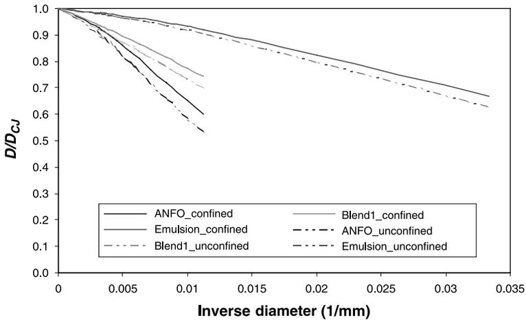
**Fig. 10.** Unconfined and confined (kimberlite)  $D/D_{CJ}$  versus diameter relations of ANFO, Blend1 and emulsion
