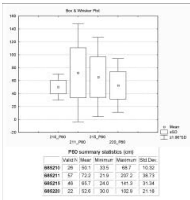
Figure 6: Fragmentation analysis of truck trays using Split Desktop.
