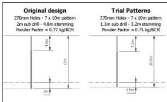
Figure 2: Benchmark and trial blast design variables.
