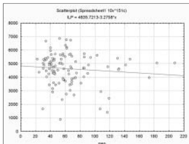
Figure 8: Instantaneous loading productivity (t/h) versus P<sub>80</sub> (cm) for all trials.
