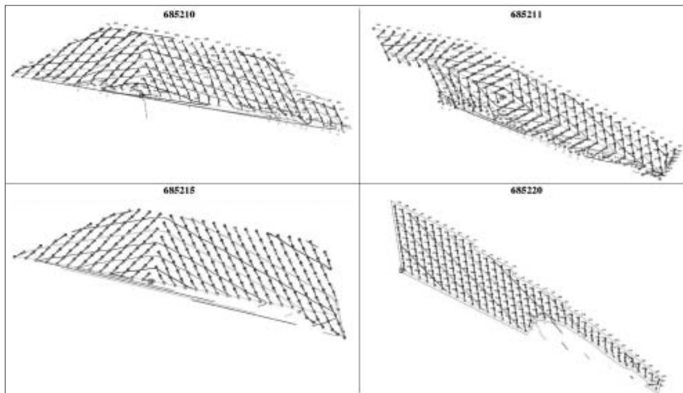
Figure 3: Shape of blast sequencing for each trial blast.
