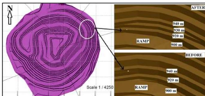
Figure 5. Geotechnical design changes at north-east section of the pit.
