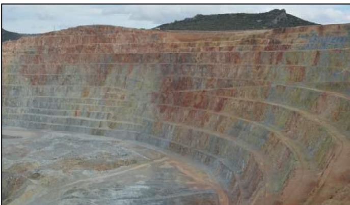
Figure 8. A view from very good single and double bench profiles with good floor conditions at Kışladağ Mine.
