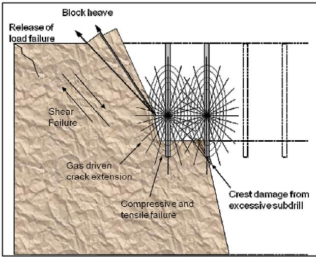
Figure 6. Blast induced wall damage mechanisms (ISEE 1998).
