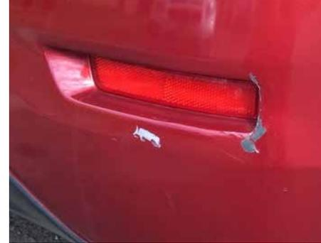
✘ Damage to the paint finish that will require repainting
