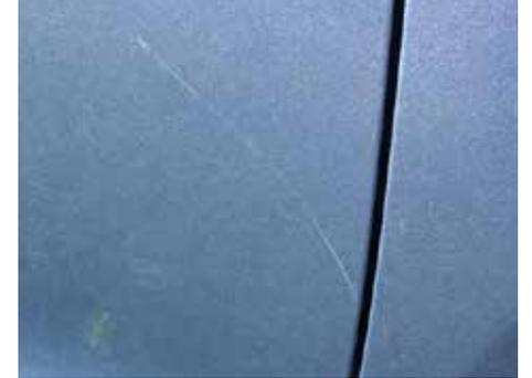
✘ Scratch has penetrated through the clear coat. Scratch exceeds 25mm
