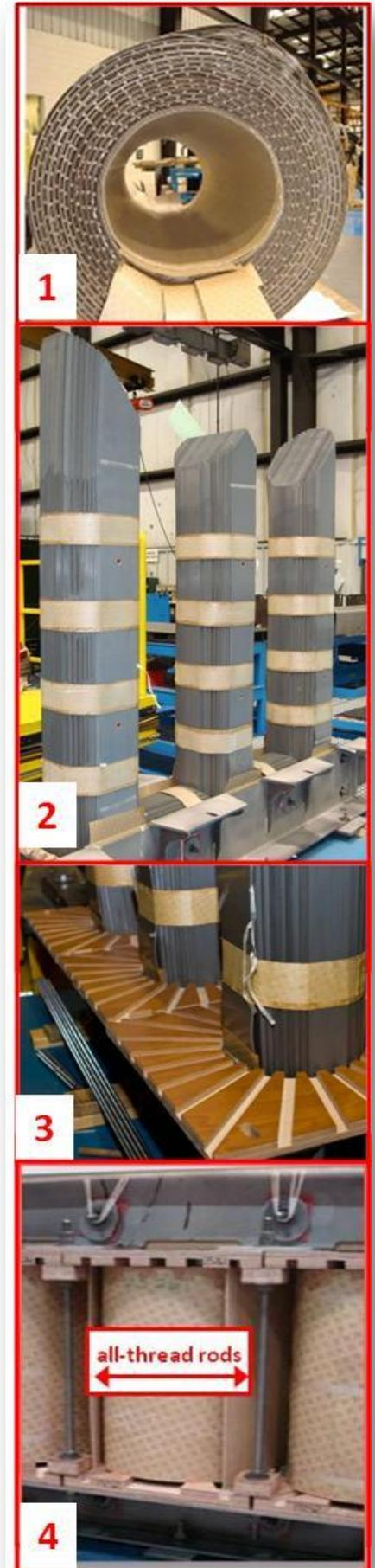
These forces must be contained to prevent telescoping of the coils which can result in short-circuited winding turns and coil failures.
