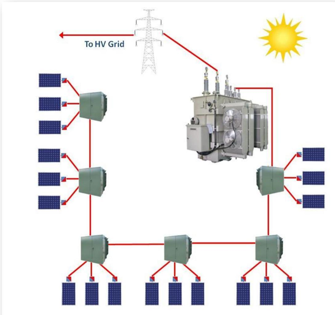
The above provides a visual as to how a solar farm utilizing multiple secondary input step-up transformers would connect the key components to the high voltage grid. Transformers with this configuration are anything but “off the shelf”. Their construction must be highly reliable, highly efficient, and must cool effectively. As technology progresses, the total kVA rating requirements are sure to rise.
