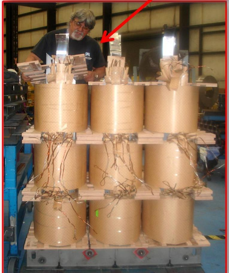
The low voltage buss-work is then added. The winding starts and finishes for each of the three transformers are wye connected complete with welded termination pads which will be bolted to the low voltage tank bushings.
