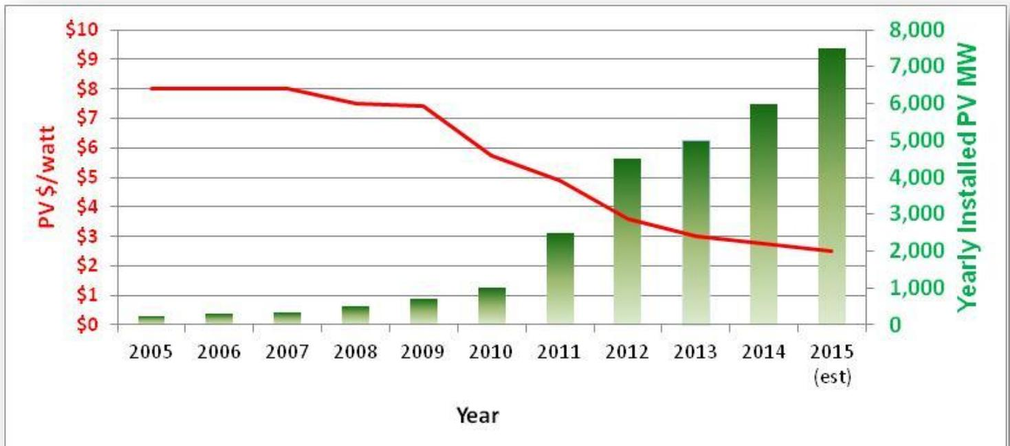
The illustration above graphs the annual U.S. production rate against the cost to produce. Production rates have actually increased by over 100 times within the the past 10 years! As is the case with wind power, the demand for solar power is well positioned to continue growing at a pace unprecidated to that of “conventional” energy alternatives (coal, gas, hydro).
