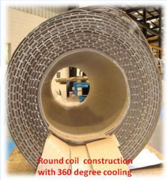
The PCT WTSU is an engineered solution that addresses the specific needs of the wind farm turbine. It reduces lost revenues due to down time and provides a lower total cost of ownership compared to standard off-the-shelf distribution transformers. Standard transformers experience frequent failures when used in wind farms, due to heat build-up from rapid and irregular thermo-cycling, frequent fault conditions, and build-up of gasses from arcing that occurs when inexpensive tap changers are used.
