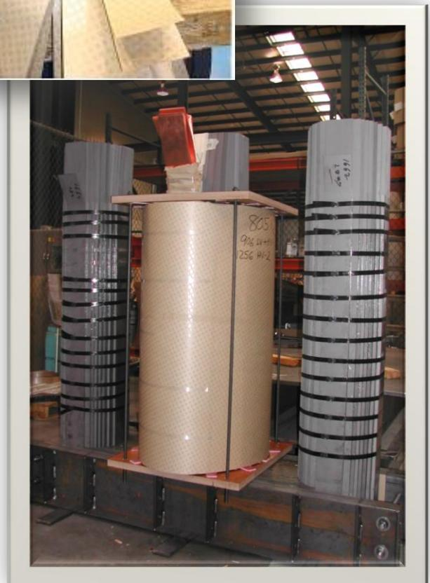
Axial forces must also be managed, especially during fault conditions. Failure to do so can lead to telescoping of the coil turns which in turn results in coil failures. Round coil construction coupled with cruciform stacked cores provide for the capability of adding pressure plates to the top and bottom of each coil.
