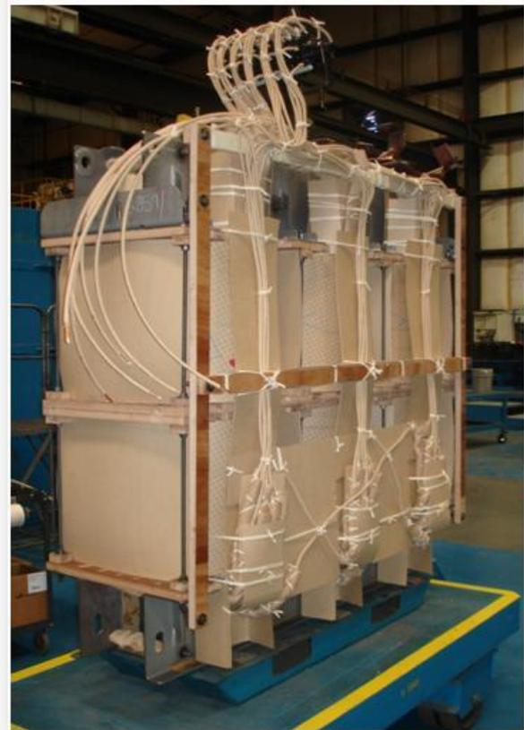
As with all products produced by Pacific Crest Transformers, strict attention is paid to the details as pertains to the application and duty cycle for each transformer provided. Specific design parameters are utilized for specific needs. There is far more to specifying a liquid filled transformer than mere kVA and voltages. Although all transformers must meet ANSI construction and test
