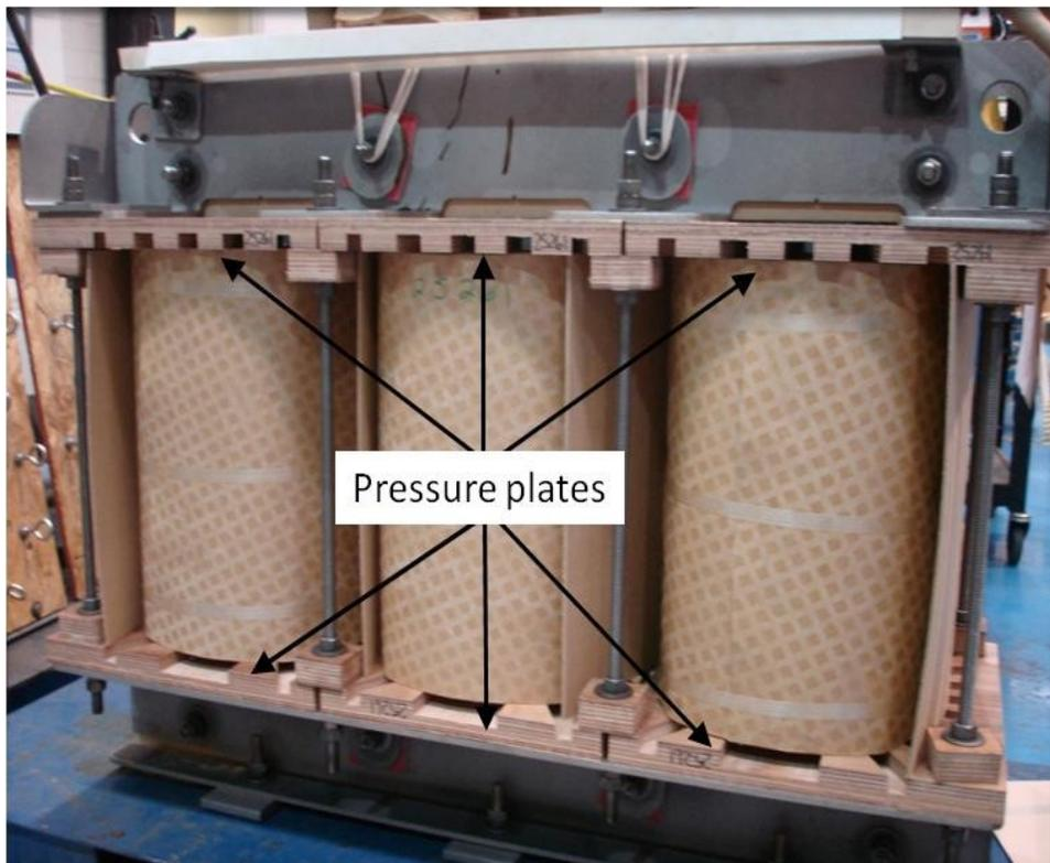
Round coil construction coupled with cruciform stacked cores provide for the capability of adding pressure plates to the top and bottom of each coil.
