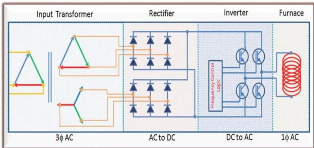
The preceding diagram is a simplified representation of the induction furnace electrical system. A 3-phase line frequency supply feeds a 3 phase transformer. The output feeds a full wave rectifier circuit which produces a DC output. Then, the DC is changed into single-phase AC via the inverter circuit. The inverter is IGBT (insulated gate bipolar transistor) based which enables precision frequency control. The variable frequency is then fed to the furnace coil.
