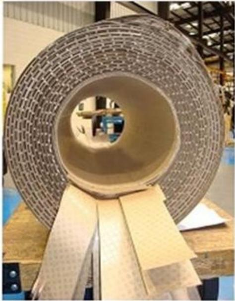
The utilization of round coils with cruciform stacked cores allows for 360 degree coil cooling thereby minimizing hot-spots. Round coils also effectively manage radial forces since they are equalized throughout the circumference of the coils. Management of coil heating and radial movement protects the winding layer insulation system from premature aging and rupture.
