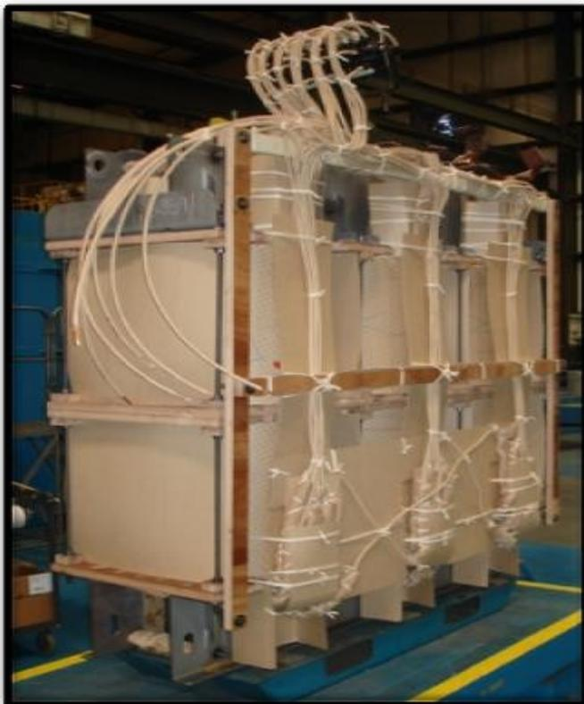
**12 pulse core/coil assembly**
