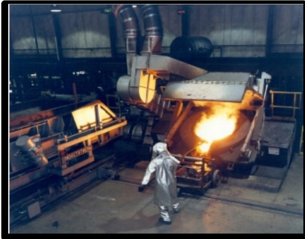
Electromagnetic induction is the process that allows an induction furnace to work. It was first discovered in 1831 by Michael Faraday. During induction, an electric current is passed through a metal coil which creates a magnetic field. When metal is introduced into the magnetic field, an electrical current passes through the metal and causes it to heat.
