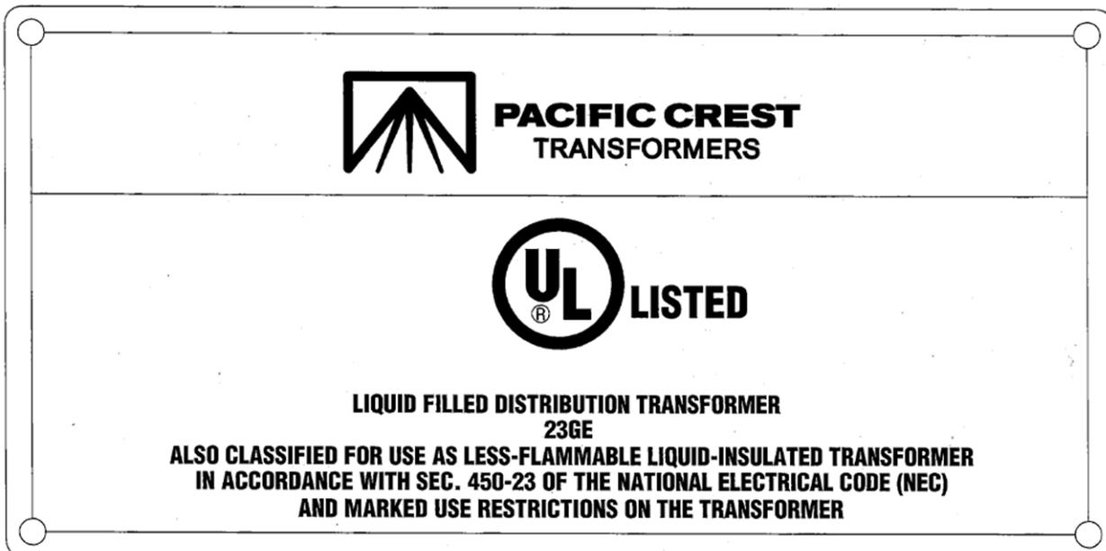
Although the means in which UL and FM approach compliance with NEC 450-23 differ, both are considered equal in their application. The FM approach uses a dedicated standard for compliance whereas UL combines a listed transformer with a classified fluid while adding the specific requirements of NEC 450-23 to achieve compliance. The net result is that both approaches provide third party compliance with NEC for indoor and outdoor transformer installations and are verifiable by the AHJ.
