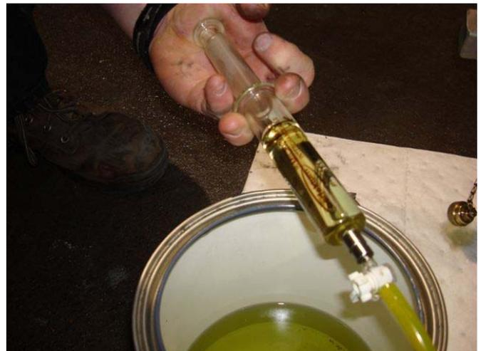
Hold backpressure against the syringe plunger as it fills to 1/16" past the last gradient mark.
