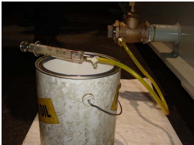
Turn three way shut off valve to allow the fluid to drain into bucket.
