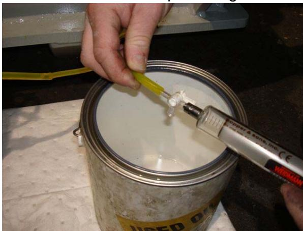
Connect hose to syringe three way valve and aim into waste bucket.
