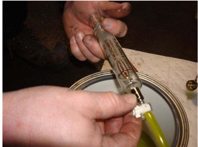
Turn valve and purge dry air from inside the syringe toward the hose end.
