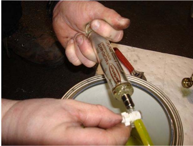
Continue to push the fluid from the syringe into the oil waste container and purge any air bubbles. Sometimes it is necessary to hold the syringe (hose end) upwards.
