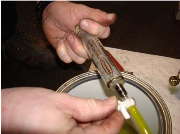
Turn valve to allow the transformer oil to begin filling the syringe. Complete this process three times(3).
