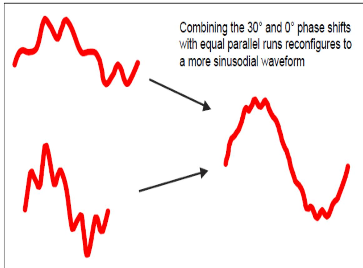
For maximum benefits from harmonic mitigating transformers, both 30° and 0° phase-shift-equivalent products should be incorporated into the system. When this is not possible due to floor space, load requirements, or economic conditions, either product can be incorporated into the system. To combine even more harmonics, the customer can add the +15° or -15° (45°) products to their application.
