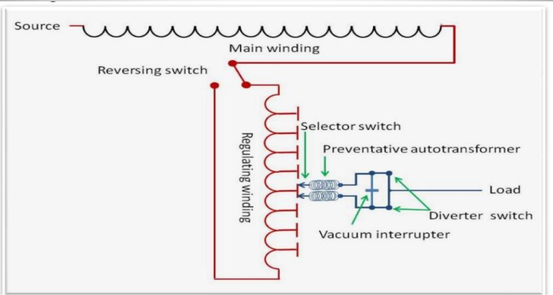
**Schematic detailing key components of LTC transformer**
