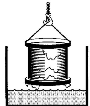
Tank is depressurized, coil is removed
