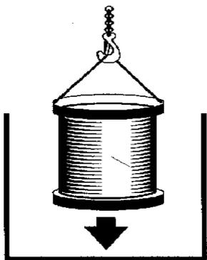
Core/Coil is put into tank
