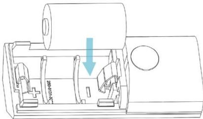
Remove the packing tape, if present, from the battery cover and install the CR2 battery with polarity as shown.
