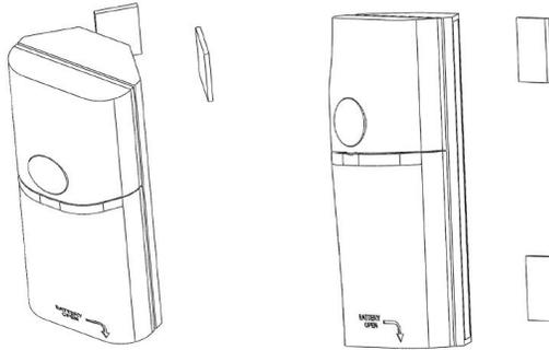
Install the Motion Sensor on a clean surface using the 2-sided tape provided. It can be installed on a flat surface or in a corner, vertically, horizontally or upside down.
