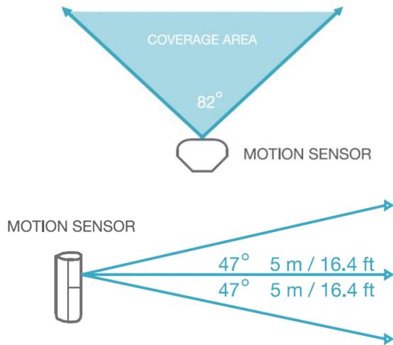
Orient the Motion Sensor for best use of its detection zones.
