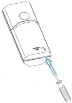
To open the battery cover, use a flathead screwdriver in the recessed slot as shown.
