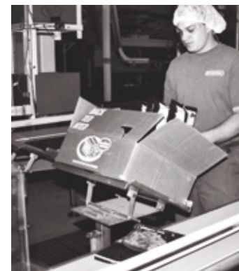
A tilted container provides the worker with easy access to the contents of the container.
