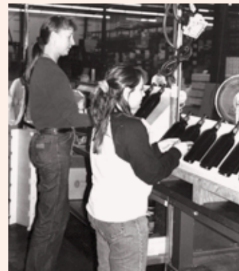
Adjustable workstations allow employees to work in a comfortable, neutral position.
