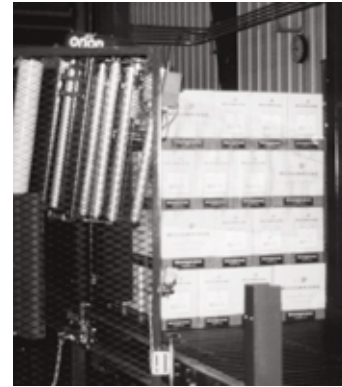
Automated shrink wrap equipment eliminates the need for workers to be in awkward postures.
