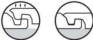
**NOTE:** Thumb pressure should be enough to engage the locking mechanism.
