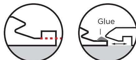
SONO planks are manufactured with Megaloc; a built-in locking mechanism that is designed to make the installation process quick and simple.
