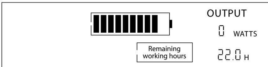
When the power is recognized to be too weak to charge the Safari LT, the display will be shown as below. This is normal, and you only need to charge with stronger sunshine or by AC power.
