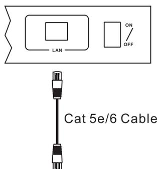
Connect to local area network router or directly to PC
