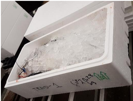
Figure 1. Fresh rainbow trout traditionally packed with ice in a 40 L EPS box with drain holes.
