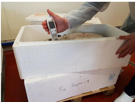
Figure 2. Superchilled rainbow trout packed without ice in an EPS box measured at -1.2 °C after 8-day transport from Iceland to Poland.
