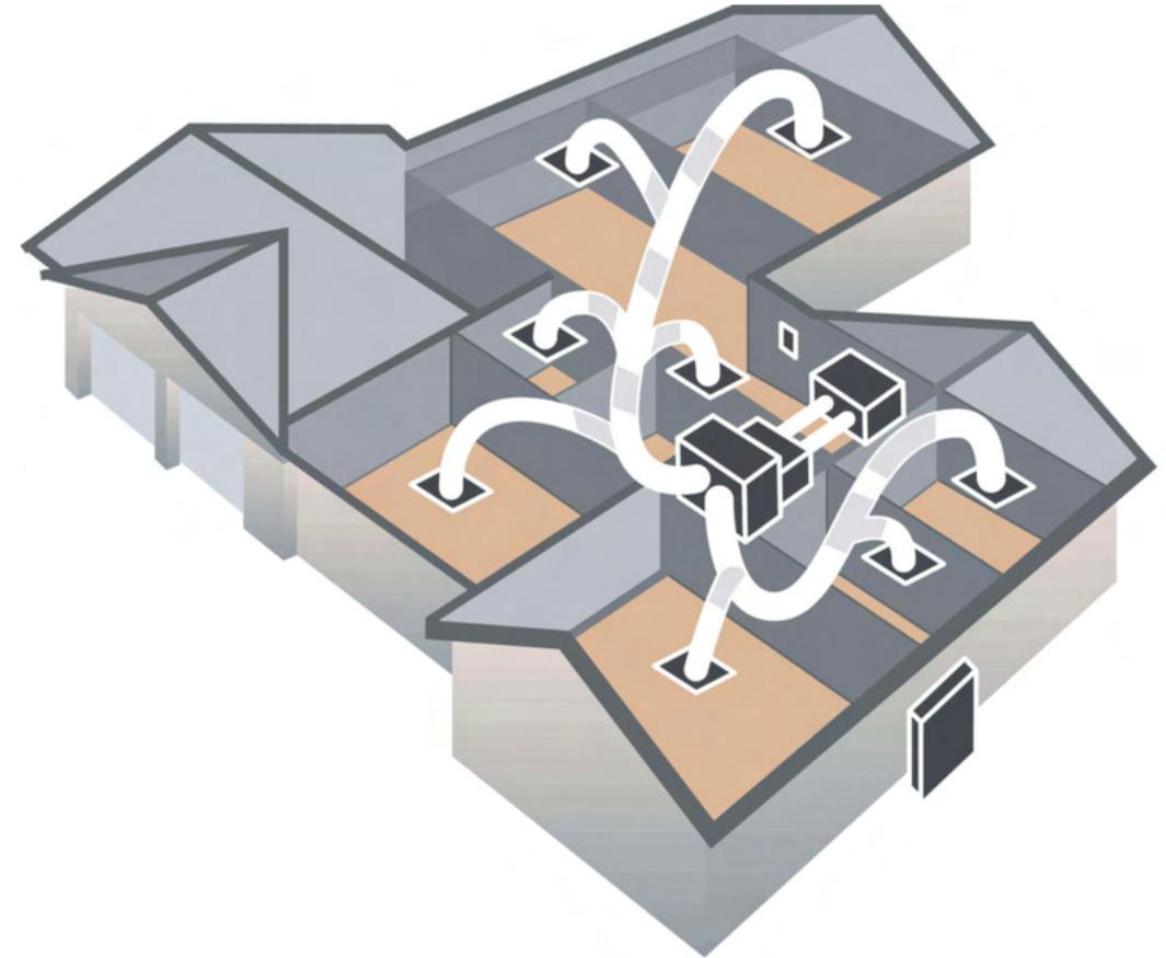
Geminair's ducted systems can be designed to operate in two or more zones. This means that the air conditioning system can be operated in the living areas during the day and in the bedrooms at night, saving money on energy costs.
