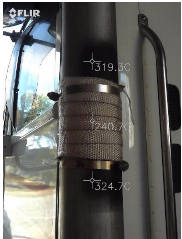
Figure 5a-b: Exhaust pipe temperature without standard heat shield taken by thermal camera with and without infra-red filter. Note that the fibreglass heat wrap, in this case, is not adequate for compliance to the standard. Shown under full engine load.
