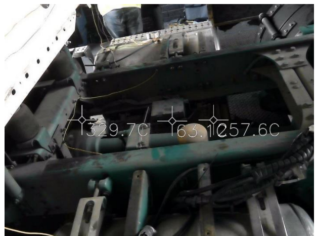
Figure 8a-b: Exhaust pipe with After Treatment Device (ATD) without heat shield taken by thermal camera. Note the ATD is double insulated in this case and does not need further shielding.
