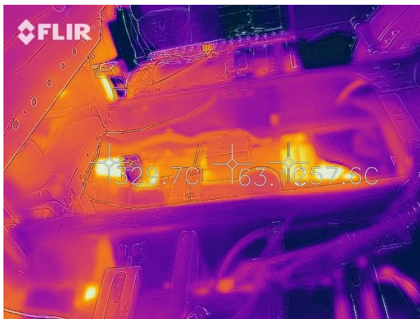
Figure 8a-b: Exhaust pipe with After Treatment Device (ATD) without heat shield taken by thermal camera. Note the ATD is double insulated in this case and does not need further shielding.
