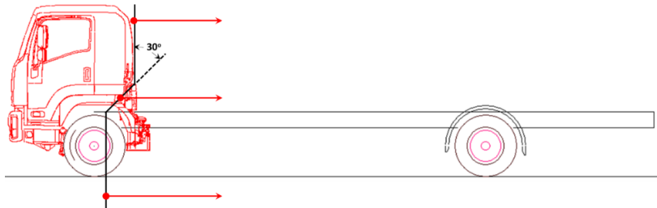
Figure 2: Example of the area where hot components must be assessed.
