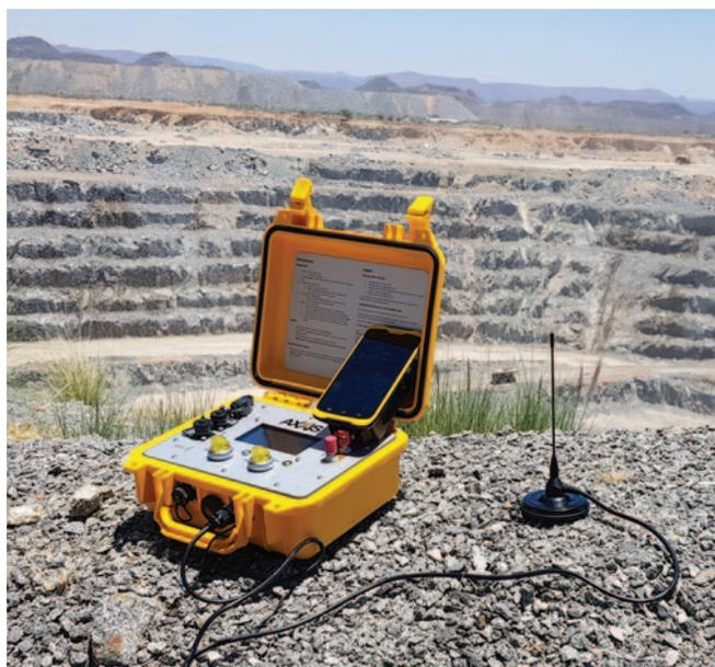
BME's latest BLASTMAP offering includes a feature to help control the shape of the muckpile, suiting it to the excavation method.
