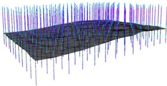
Figure 2. DataCloud's hardware RHINO, and software MinePortal, combination developing a coal model that clearly depicts the top of a coal seam.
