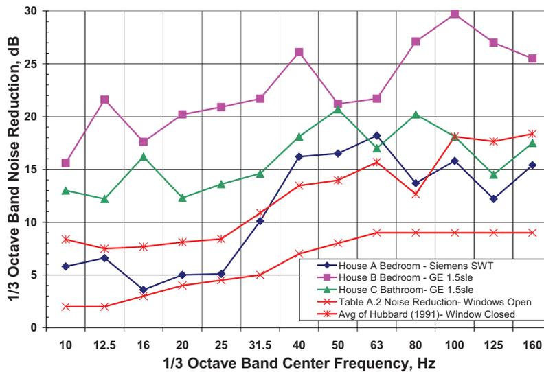
Fig. 19—One-third octave band interior noise reduction—Windows closed.
