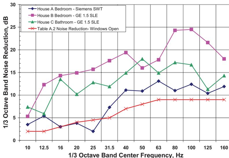
Fig. 20—One-third octave band interior noise reduction—Windows open.
