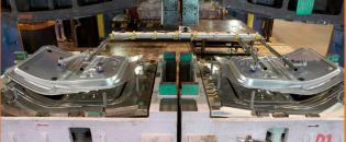
**Press Line.** The press line is fully mechanised with robots that feed the blank between the presses. The line can be operated at 1–6 stages with output after each stage. The press line can also be run in reverse, that is to say with input from press 6.
