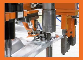
**Roller Hemming.** EBP roller hems both steel and aluminium, in both the flex-line and in flexible stand-alone cells. Roller hemming is used primarily for smaller production volumes, in series production as well as for aftermarket operations.
