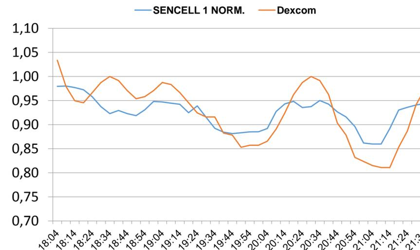
Fig.3.: Raw data signal of the Sencell device after retrospective one-point calibration with the Dexcom G4 sensor
