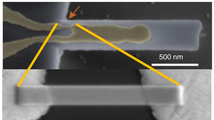
Fig.4.: Manufacturing of the nanosensors by means of the 3D-Nanosense® printing process (CantiMed)
